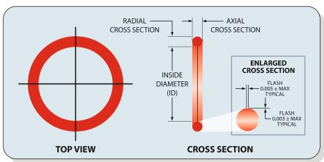
O RINGS ARE MANUFACTURED ACCORDING TO VARIOUS INTERNATIONAL STANDARDS VIZ. AS568 A, DIN 3771, BS 1806, SMS 1586, METRIC, JIS 2401, AMS, NAS, CUSTOM STANDARDS ETC.
